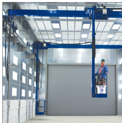
Overhead Lift System with Drop-Down Platform
